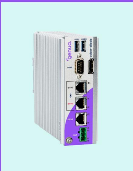
cyber-diode supports the Industry 4.0 protocol Unified Architecture (OPC UA). This is an open standard to exchange machine data.
